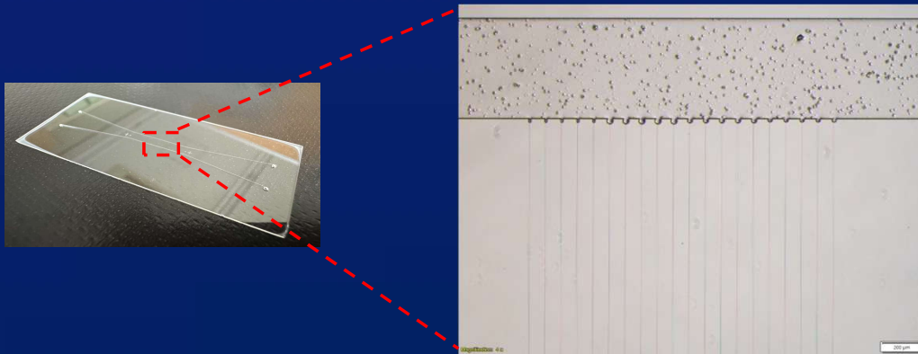
Microchannel/single cell chamber/nanofluidic channels on glass
